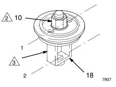
**NOTE:** Opposite holes (center line 1) must be parallel to yoke (Center line 2)
