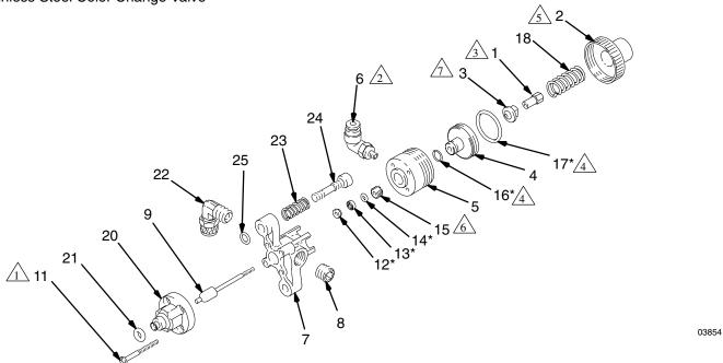
Torque screws (11) oppositely and evenly to 3–5 in-lb (0.34–0.56 N•m). If leakage occurs, torque to 8 in-lb (0.91 N•m) maximum.
