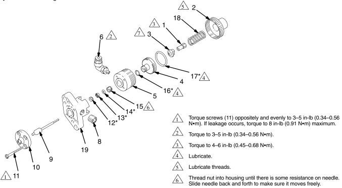
then back the retainer off 1-1/2 turns. Part No. **Description** Part No. **Description** Ref. Qty. Ref. Qty. No. No. SCREW, machine, pan 1 180537 NUT, retainer; M2.5 x 0.45 1 11 108018 4 head; M3 x 0.5 mm mm 180612 12\* SPACER, packing; Delrin CAP, retaining 1 178763 1 RETAINER, piston; M2.5 x 180539 1 13\* 178409 PACKING, fluid, UHMWPE 1 0.45 mm 14\* O-RING; Viton® 168518 1 180538 **PISTON** 1 15 180542 NUT, packing; M8 x 1 mm; 1
