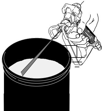
5. Trigger gun into grounded metal bucket.
