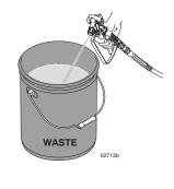
14 Point spray gun into waste pail. Squeeze spray gun trigger. Release spray gun trigger when paint comes out of spray gun.
