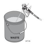
Point spray gun into waste pail. Squeeze spray gun trigger. Release spray gun trigger when paint comes out of spray gun.
