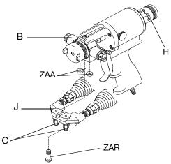
Fig. 12 Coupling Block
