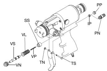
Fig. 21 Replace Trigger Valve O-Ring
