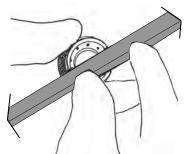
Fig. 22 Unthread Cap from PDC Body
