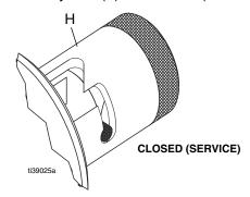
3. If attached, turn both manual valves (C) fully clockwise to close
