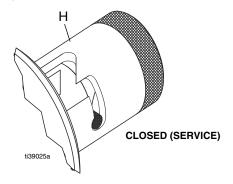
8. Remove the mixing module retainer (ZAM).
