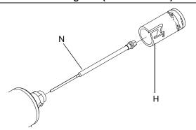
Fig. 19 Remove Valving Rod (GX-7A and GX-7 400 models)
