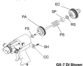
Fig. 20 GX-7 DI End Cap and Air Piston Assembly
