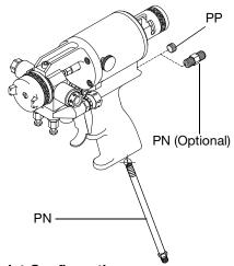
Fig. 13 Air Inlet Configurations
