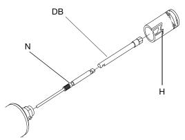
Fig. 18 Remove Valving Rod (GX-7 DI model)
