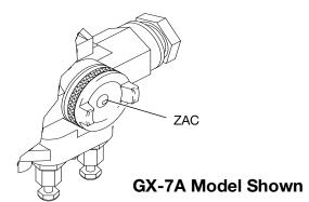
Fig. 25 Clean Pattern Control Disc
