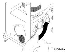
d. Install IEC connector and tighten cord clamp. Install air hose to outlet fitting. Make sure cord is pushed in as far as it will go to ensure a good connection.
