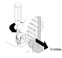
b. Remove air hose from compressor and remove outlet fitting from compressor.
