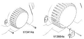
b. Install air outlet fitting.
