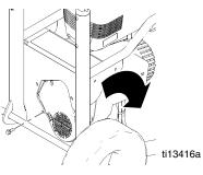
d. Remove two screws and IEC cord clamp. Remove two screws and compressor shroud.
