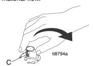
**NOTE:** Fine flow rate adjustments can be made using "+" and "-" buttons on inline valve controller. Flow rate can only be adjusted relative to position of flow control knob. The fine flow rate can only go down from, and up to the flow control knob setting.
