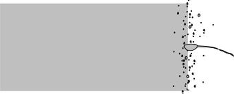
ti15525a                    | Excess material has accumulated on Spray Tip/Guard Assembly. | See <b>Shutdown and Cleaning</b> , page 17.                   |
