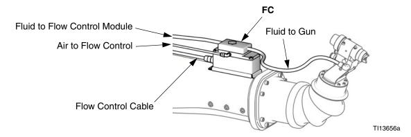
Fig. 1, 249849 Flow Control Module
