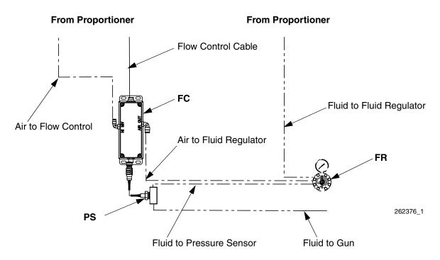
Fig. 2. 24H989 Flow Control Module, with Remotely Mounted Fluid Regulator
