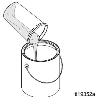
6. Insert a new liner into cup and fill 1/2 full with appropriate flushing fluid. Screw on lid and attach cup to sprayer. Shake sprayer to move flushing fluid around and clean all wetted areas inside cup.
