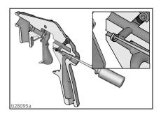
Push new seal (4) in place using a small diameter (1/4 in. or smaller) object.
