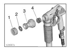
For Standard operation: install nozzle
