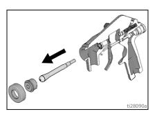
2. Use a hook-shaped object to carefully pull up-cup retainer and u-cup out of gun.
