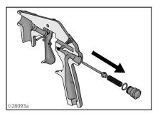
2. Use a hook-shaped object to carefully pull u-cup seal (4) out of gun.
