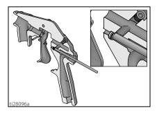
4. Replace air valve needle (17) seal (18), spring (19) and O-ring (20) if necessary.
