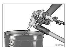
Remove nozzle from gun. Trigger gun into bucket until most of texture mix is pumped out. Allow water to flow through gun until gun is clean.
