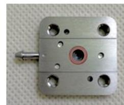
**Note:** When installing the nozzle, the o-ring must face *up*.
