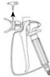
REMOVE SPRAY TIP. ENGAGE GUN SAFETY LATCH.
