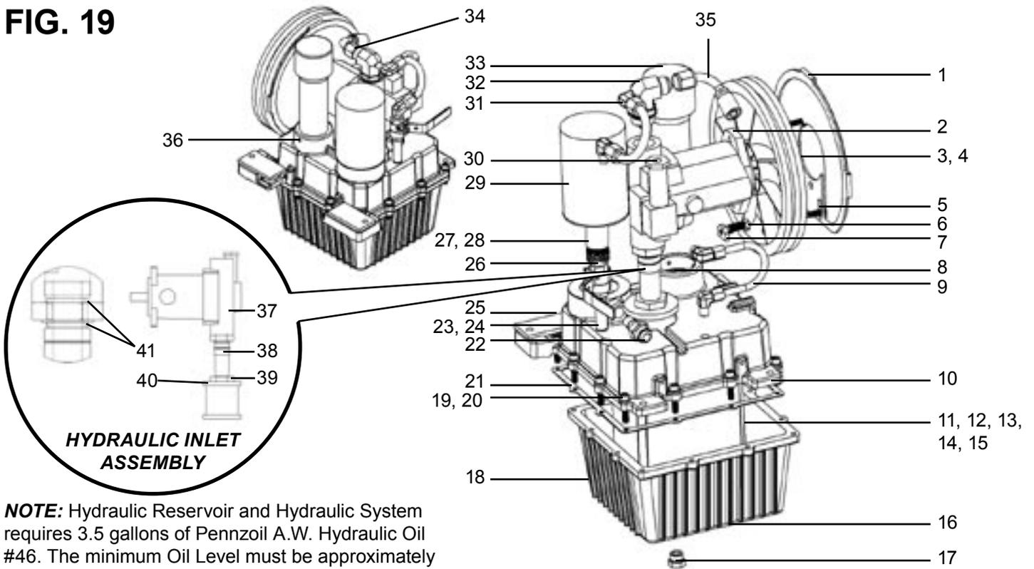
**NOTE:** Hydraulic Reservoir and Hydraulic System requires 3.5 gallons of Pennzoil A.W. Hydraulic Oil #46. The minimum Oil Level must be approximately halfway up the Filler Tube. Never below.
