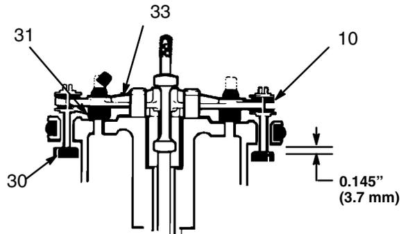
7. Install the transfer valve grommets (10), then reassemble the valve mechanism. Before installing the lockwires (13) in the adjusting nuts (11), use the special gauge, 171-818, to adjust the transfer valve so there is 0.145 in. (3.7 mm) clearance between the poppets (30) and the seat when it is open. See Fig 11-1. Snap the toggles (15) to the up position.
