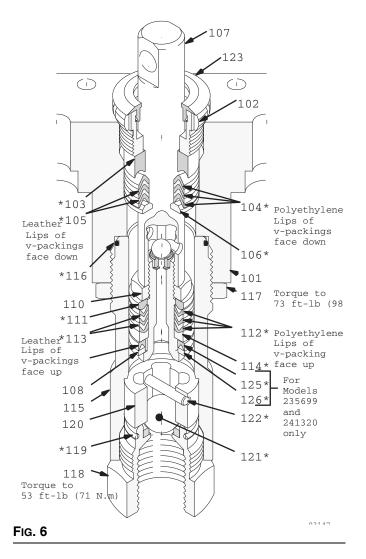
10. Install the packing nut (102) and plug (124), but leave loose for now. See Fig 7.
