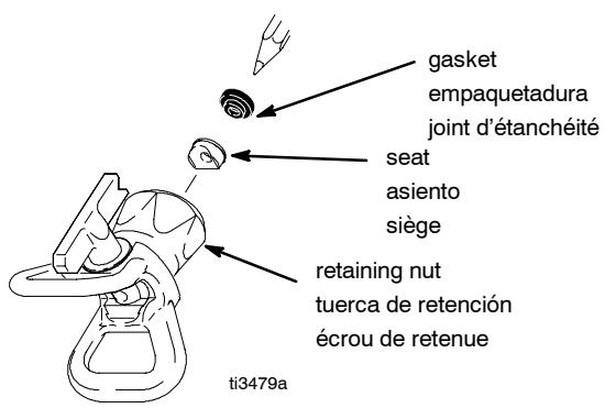
1. Orient seat so curved face matches tip cylinder profile.
