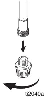
11. Connect garden hose to suction tube with Power Flush attachment. Leave prime tube in waste pail.
