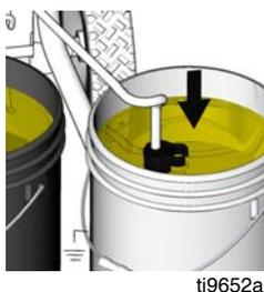
7. Submerge suction tube in water or flushing solvent.
