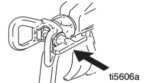
3. Screw tip and guard assembly on gun. Tighten retaining nut.
