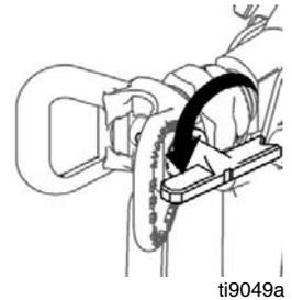
Point the arrow-shaped handle on the spray tip forward to SPRAY and backward to UNCLOG obstructions.
