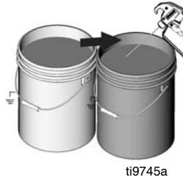
18. Stop triggering gun. Engage trigger lock.
