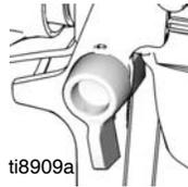
**NOTE:** Some fluids may prime faster if the Power Switch is momentarily turned off so the pump can slow and stop. Repeat several times if necessary.
