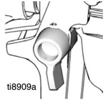
5. When obstruction is cleared, engage trigger lock and rotate arrow-shaped handle back to SPRAY position.
