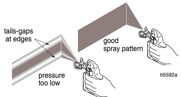
If tails persist when spraying at the highest pressure, a smaller tip is needed or the material may need to be thinned.
