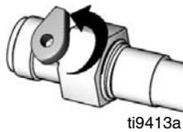
8. Turn on water. Open valve. Rinse paint off suction tube, prime tube and inlet screen.
