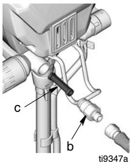
4. Tighten outlet fitting and reconnect hose (a) to sprayer. Use two wrenches to tighten securely.
