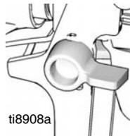
16. Transfer prime tube to paint pail and clip prime tube to suction tube.
