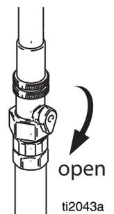
14. Circulate water through sprayer, into waste pail, for 20 seconds.
