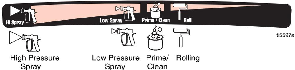
To select function, align symbol on pressure control knob with setting indicator on sprayer.
