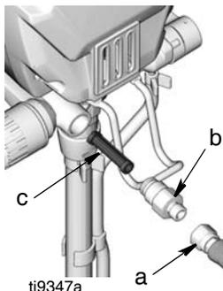
3. Check InstaClean Fluid Filter (c) for debris. If needed, clean filter with water and a soft brush.
