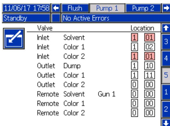
Figure 57 Pump Screen, Valve Assignment with duplicates
