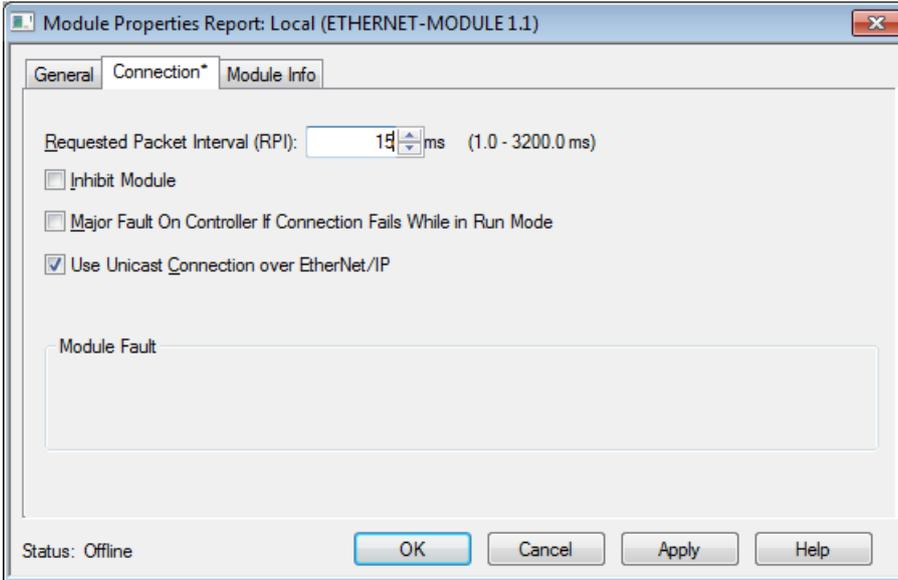
**NOTE:** An asterisk appears after the tab heading if unsaved changes are present. Click the Apply button to save changes without exiting this screen.
