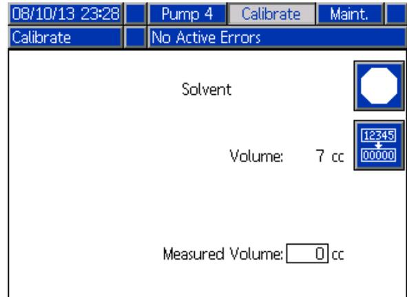
Figure 70 Enter Measured Volume of Solvent
