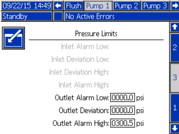
Figure 63 Pump Screen 3, Pressure Monitoring Disabled
