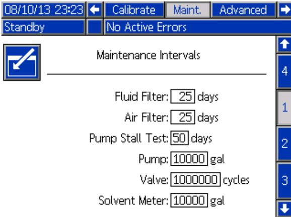
Figure 72 Maintenance Screen 1, Interval Settings
