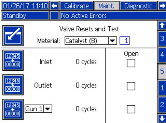
Figure 98 Maintenance Screen 5 Common Catalyst
