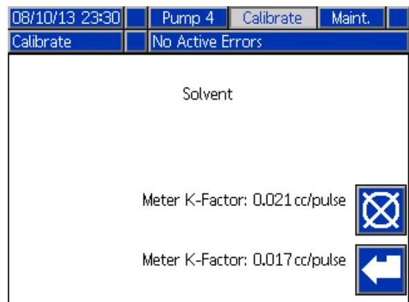
Figure 71 Accept Calibration
