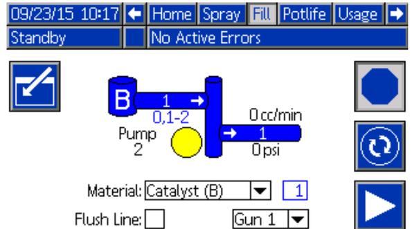
Figure 95 Fill Screen Common Catalyst
