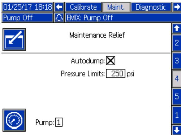
Figure 75 Maintenance Screen 4, Manual Pump Relief
