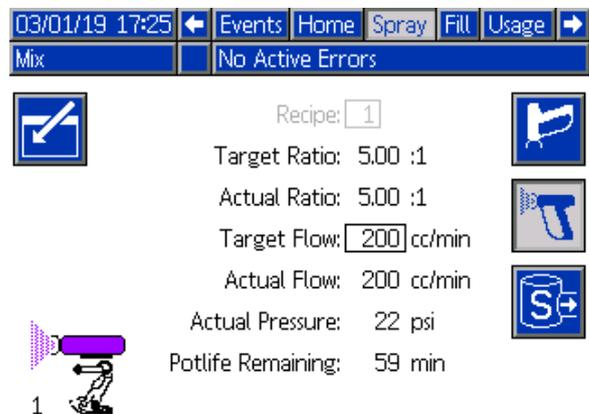
Figure 24 Spray Screen, in Mix Mode, Solvent Push Enabled
