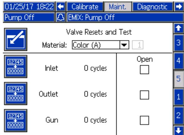
Figure 76 Maintenance Screen 5, Color Valve Resets
