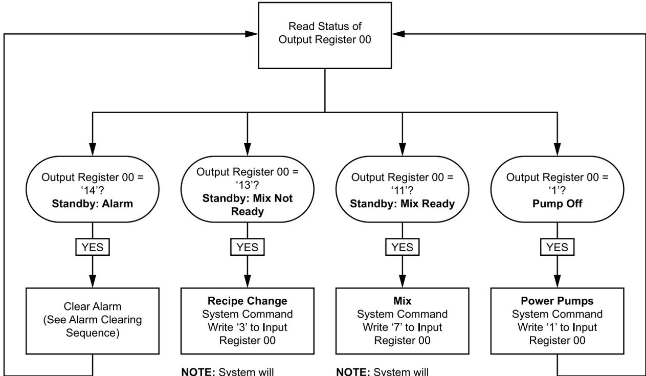
**NOTE:** System will automatically run through necessary recipe change steps based on it's current state. If **Goto Recipe Number** has not changed, it does not have to be rewritten here.
