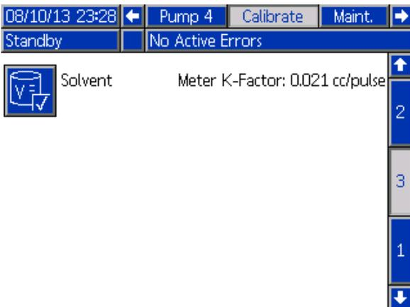
Figure 69 Calibrate Screen 3
