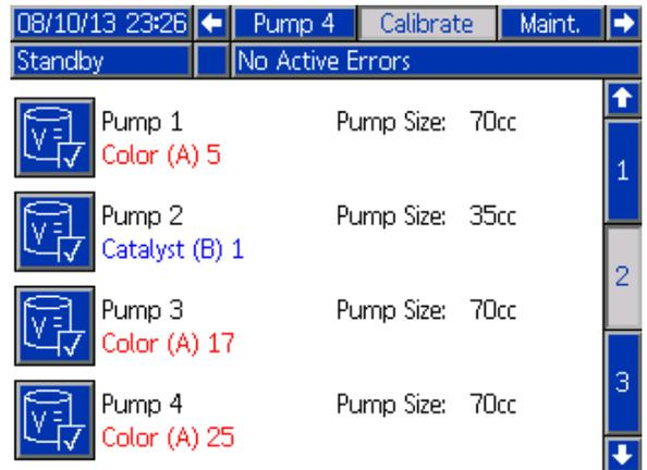
Figure 67 Calibrate Screen 2
