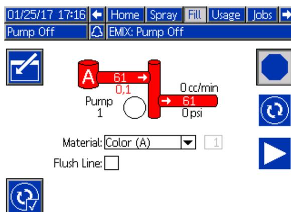
Figure 27 Fill Screen, Pre-Fill Pump Option
