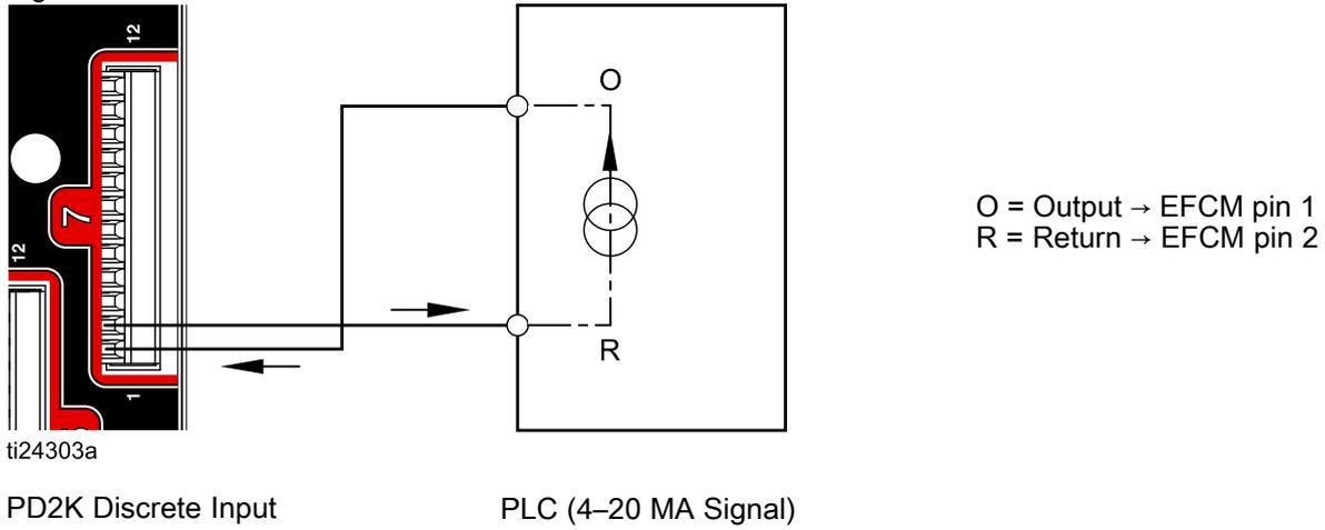
Discrete I/O Connections on EFCM
