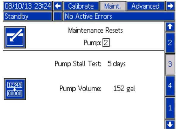
Figure 74 Maintenance Screen 3, Current Pump Status
