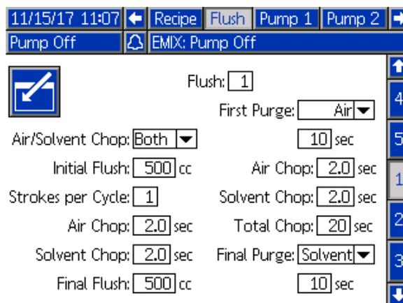
Figure 60 Flush Screen with both air/solvent chops
