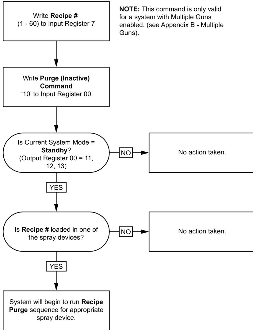
Inactive Pump Flush and Prime Sequences
