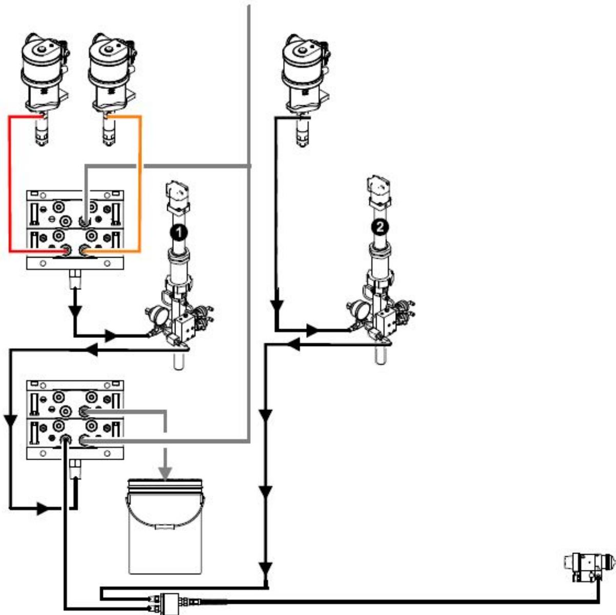
Figure 39 MISO Fluid Stream Configuration (for Solvent Push)
