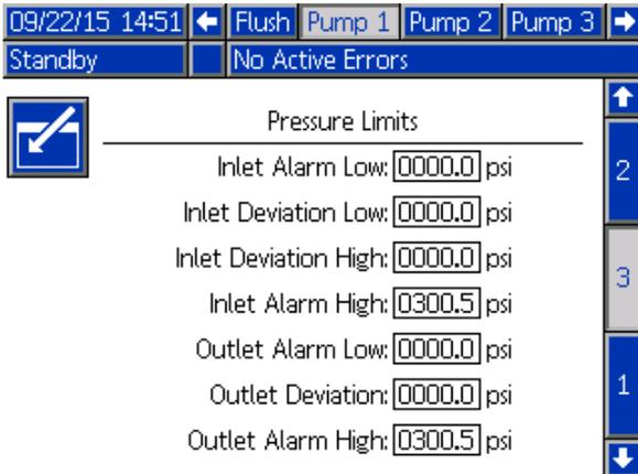
Figure 64 Pump Screen 3, Pressure Monitoring Enabled
