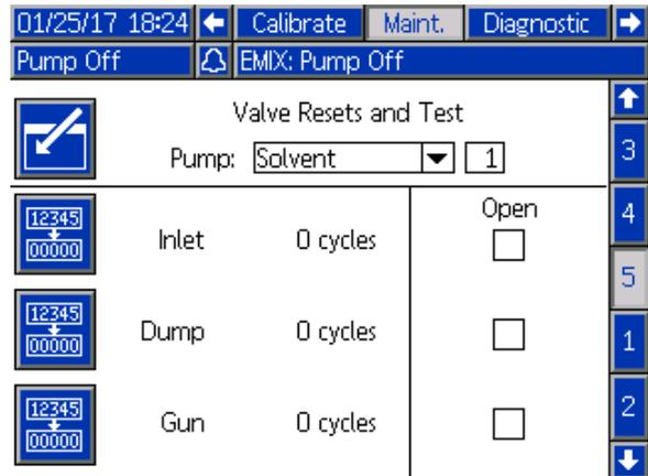
Figure 77 Maintenance Screen 5, Solvent Valve Resets
