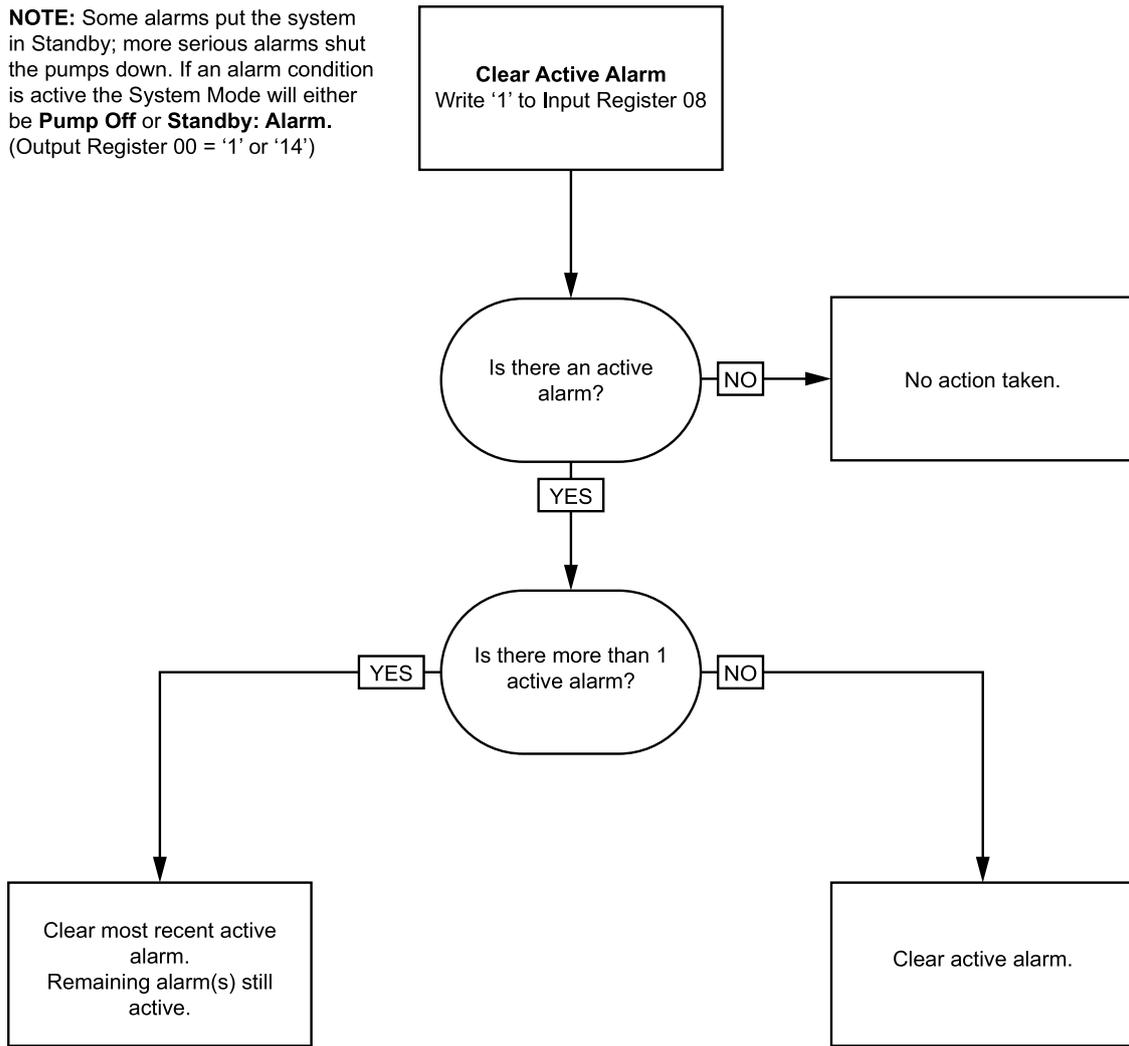
**NOTE:** If more than 1 active alarm exists a repeated write of '1' to Input Register 08 is required for each.
