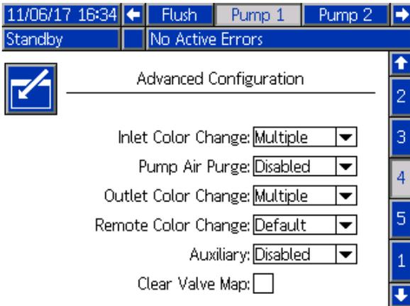
Figure 53 Pump Screen, Advanced Configuration
