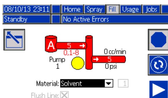
Figure 26 Fill Screen, Solvent Selected
