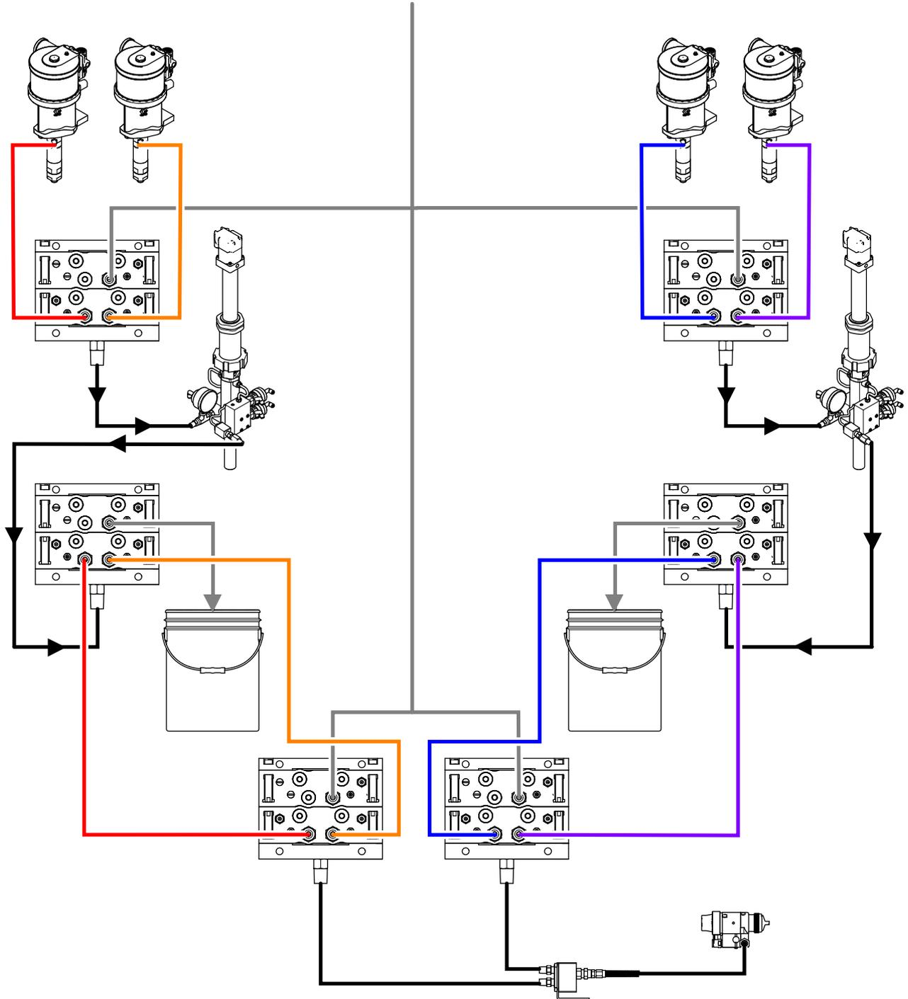
Figure 88 Fluid lines for a typical PD2K Automatic system.
