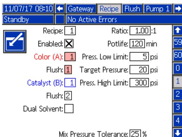
Figure 58 Recipe Screen with invalid valve location
