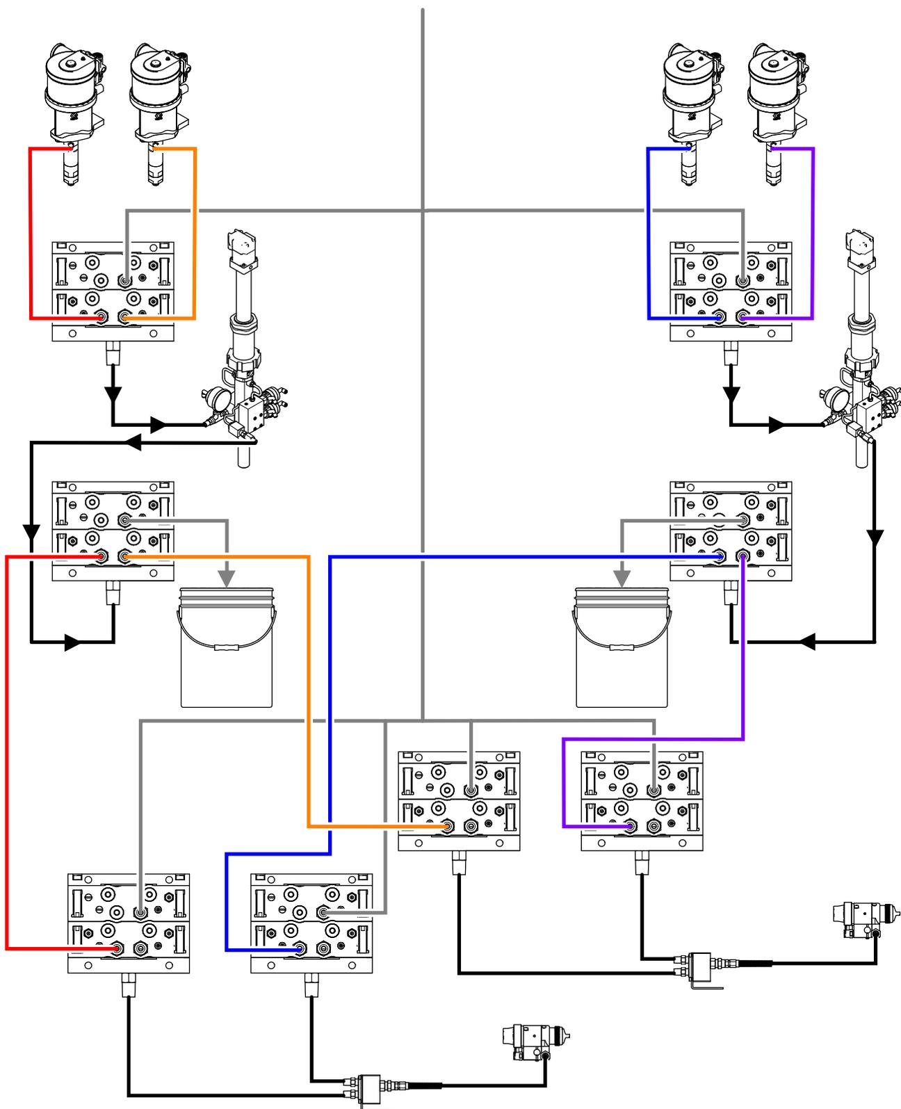
Figure 89 Fluid lines for a PD2K Automatic system with multiple guns.
