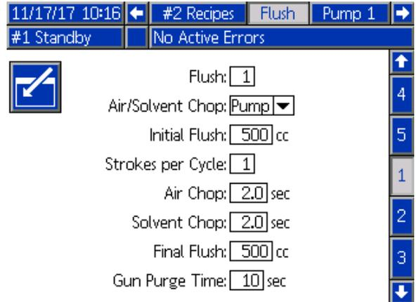
Figure 61 Flush Screen with pump air/solvent chop
