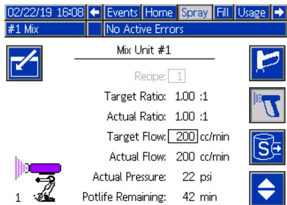
Figure 23 Spray Screen, in Mix Mode, Solvent Push Enabled
