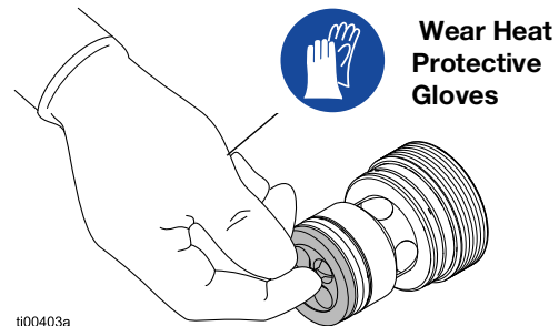
FIG. 85: Check Seat Installation Tip
