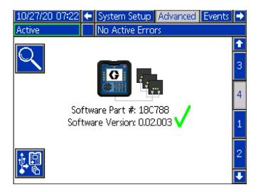
This screen can be used to view the version of software used in the system. Additionally, this screen is used to update the system software using a USB drive with the latest software and a Graco black token. The latest software is provided on Help.graco.com. Refer to the ADM Token In-System Programming manual for a detailed description of this screen. See **Related Manuals** on page 3.
