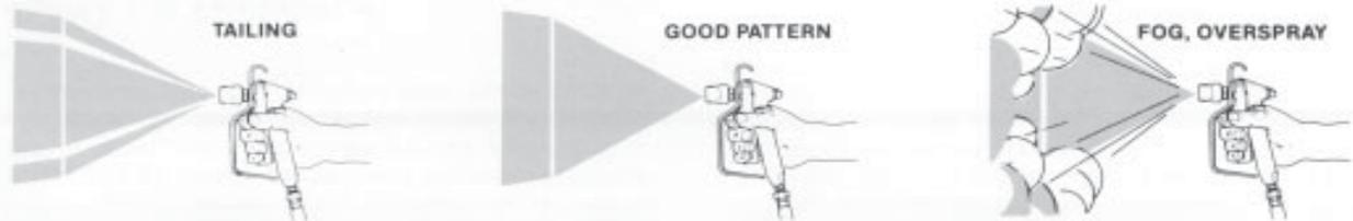
Adjust pressure control knob so that paint is completely atomized from the spray gun. Insufficient pressure will result in "tailing".
