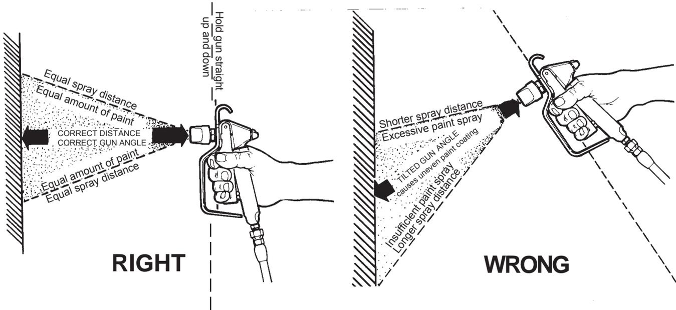
Hold the spray gun 12 - 15 inches away from the work surface and keep it perpendicular (straight) to the surface. Move the spray gun parallel to the work and at a right angle to the surface.
