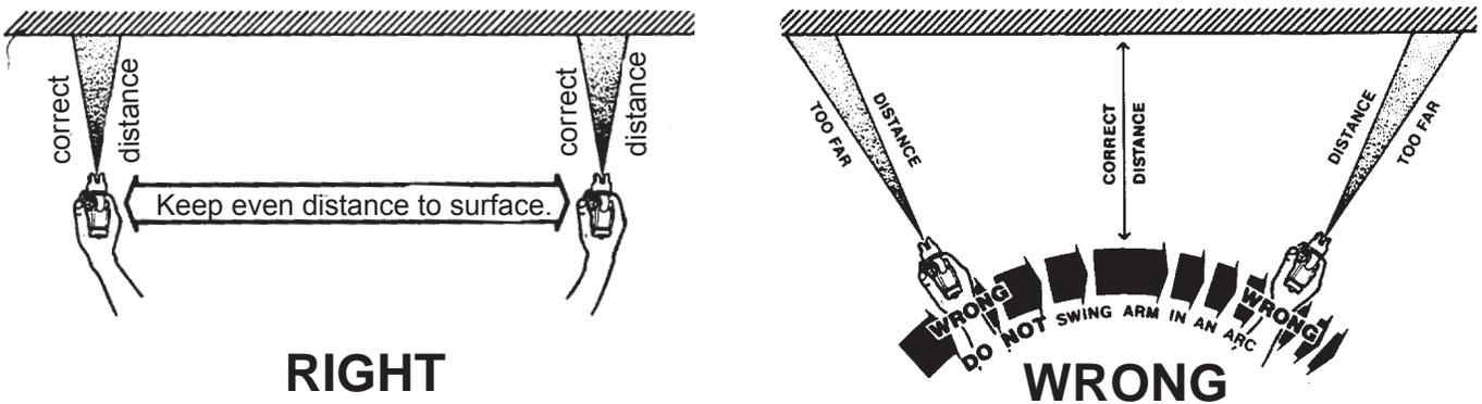
Move the gun at a steady rate in order to apply a good coverage. The wet coat should be just under the thickness at which a run or sag will occur. Slow gun movement or gun held too close will result in an overly wet or thick wet or thick coat coverage that is likely to run or sag.
