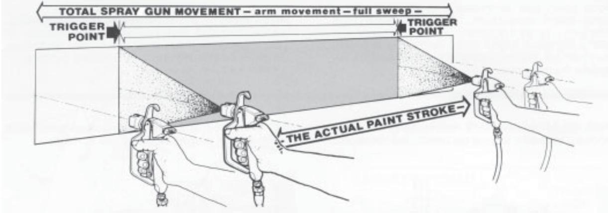
It is important to "trigger" the gun after gun movement (arm movement) has started and release trigger (shut gun off) before gun movement ends. Gun movement is always longer than actual paint (spray) stroke. In that manner, even blending and uniform paint coat thickness is achieved over the entire surface. When the gun is in motion as the trigger is pulled, it deposits an even amount of paint.
