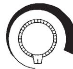
**PRESSURE CONTROL KNOB** is used to adjust pressure. Turn clockwise (CW) to increase pressure and counterclockwise (CCW) to decrease pressure.
