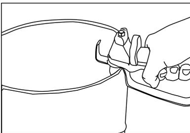
If the **SPRAY TIP OR HOSE IS CLOGGED**, follow Step 1 through 5 above. Expect paint splashing into the bucket while relieving pressure during Step 4.
