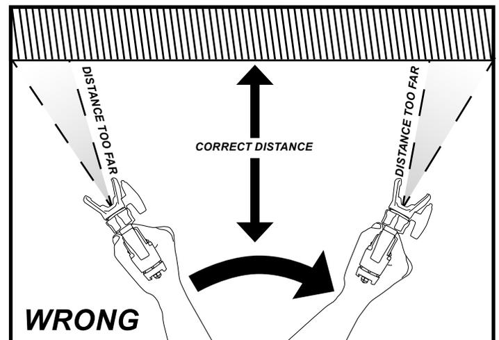
Move the gun at a steady rate in order to apply a good coverage. The wet coat should be just under the thickness at which a run or sag will occur. Slow gun movement or gun held too close will result in an overly wet or thick wet or thick coat coverage that is likely to run or sag.
