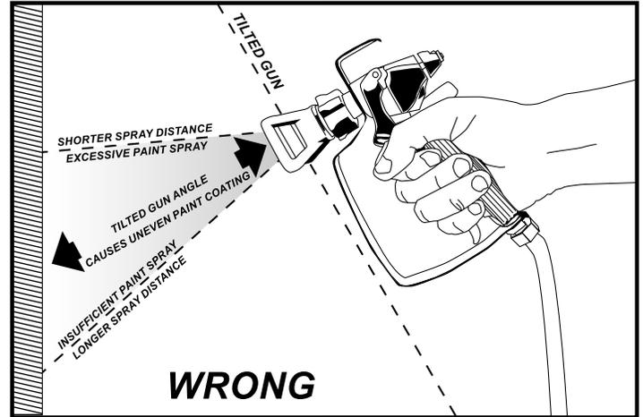
Hold the spray gun 12 - 15 inches away from the work surface and keep it perpendicular (straight) to the surface. Move the spray gun parallel to the work and at a right angle to the surface.
