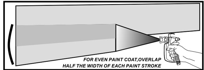
Overlap the previous pass by half the width of the spray pattern. Aim at the bottom of the previous pass.
