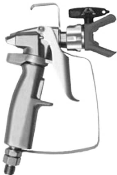
The Allpro Pro-Plus flat handle gun is designed to be very light-weight for all day user comfort. Features include a thumb actuated trigger safety lock and easy-clean filter. The extra large, 3/16" tungsten carbide ball and seat provide BOTH long wear and allow the Prolight gun to be used with heavy materials. Uses durable stainless steel (not aluminum) threads for tip attachments and its compact size provides ease of use in tight spaces such as inside cabinetry.
