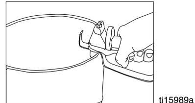
4. Re-engage gun trigger lock and turn Prime Valve to the open (priming) position.
