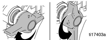
**NOTE:** The valve handle can move both clockwise and counter clockwise and can face different directions.
