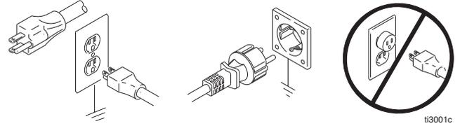
Do not modify the plug provided; if it does not fit the outlet, have the proper outlet installed by a qualified electrician.
