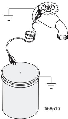
**To maintain grounding continuity when flushing or relieving pressure:** hold metal part of spray gun firmly to side of a grounded metal pail. Then trigger gun.
