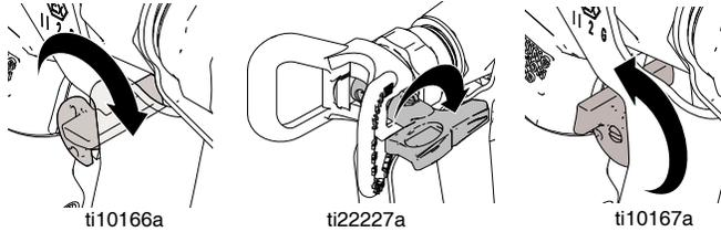
2. Engage trigger lock. Return Spray Tip to original position. Disengage trigger lock and continue spraying.
