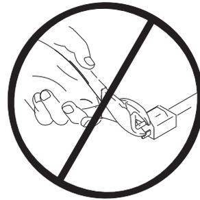
**Extension Cords:** Use an extension cord with an undamaged ground contact. If an extension cord is necessary, use a 3-wire, 12 AWG (2.5 mm<sup>2</sup>) minimum.
