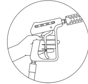
The quick connect nozzle assembly should be disconnected from the gun/wand assembly at this time by retracting the locking ring on the quick-connect fitting to remove the nozzle.
