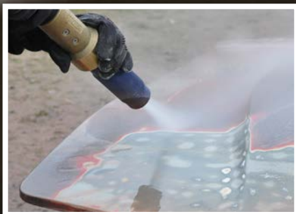
Coating and Paint Removal
