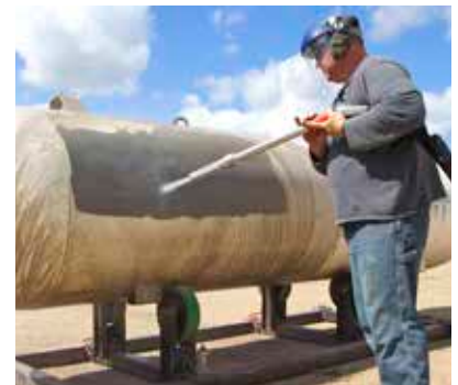
Vapor Abrasive Blasting reduces the amount of dust by up to 92%.
