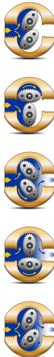
**Figure 2:** Fluid flow is shown in the **oval gear flow meters** in the figure above. The flow meter has two oval-shaped gears. The rotation of the gears traps a precise amount of fluid between the gears and the housing. By monitoring the number of gear rotations, liquid flow rate is calculated.
