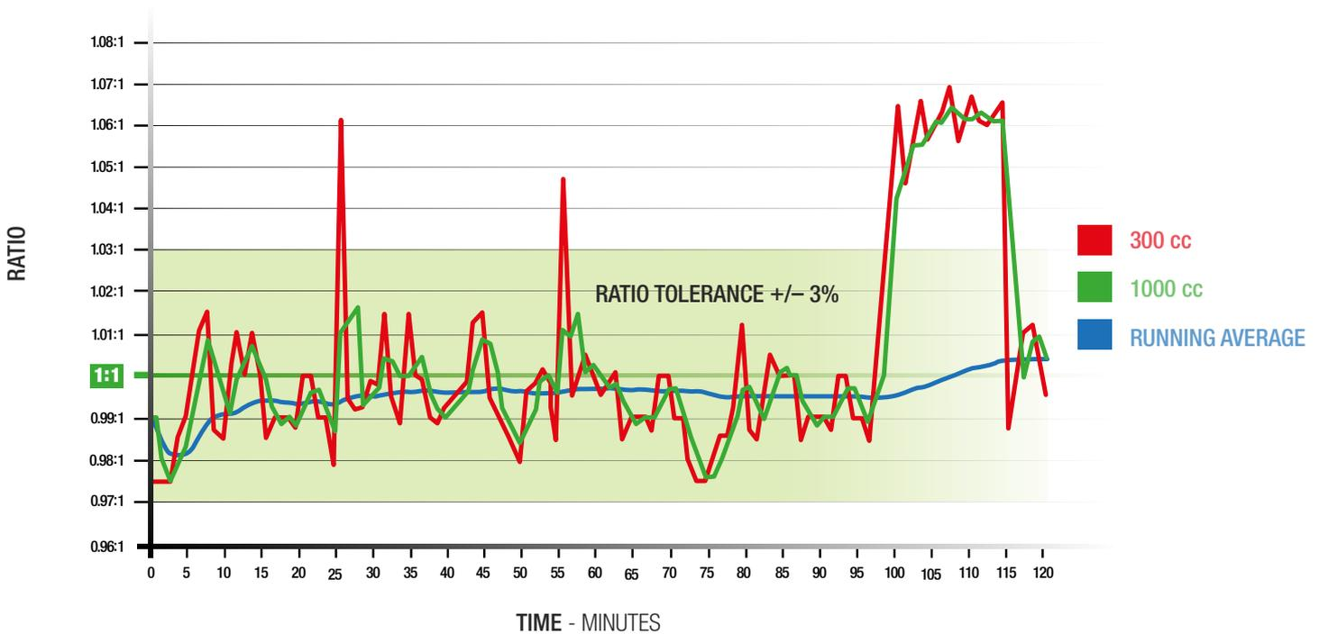
**Figure 3:** Graph shows the importance of selecting the correct volume to measure ratio. The same data is displayed calculating the ratio using 3 different volumes: 300cc, 1000cc, and a running average. At 300cc there would have been a few nuisance alarms but using a running average would not have detected a true ratio issue.
