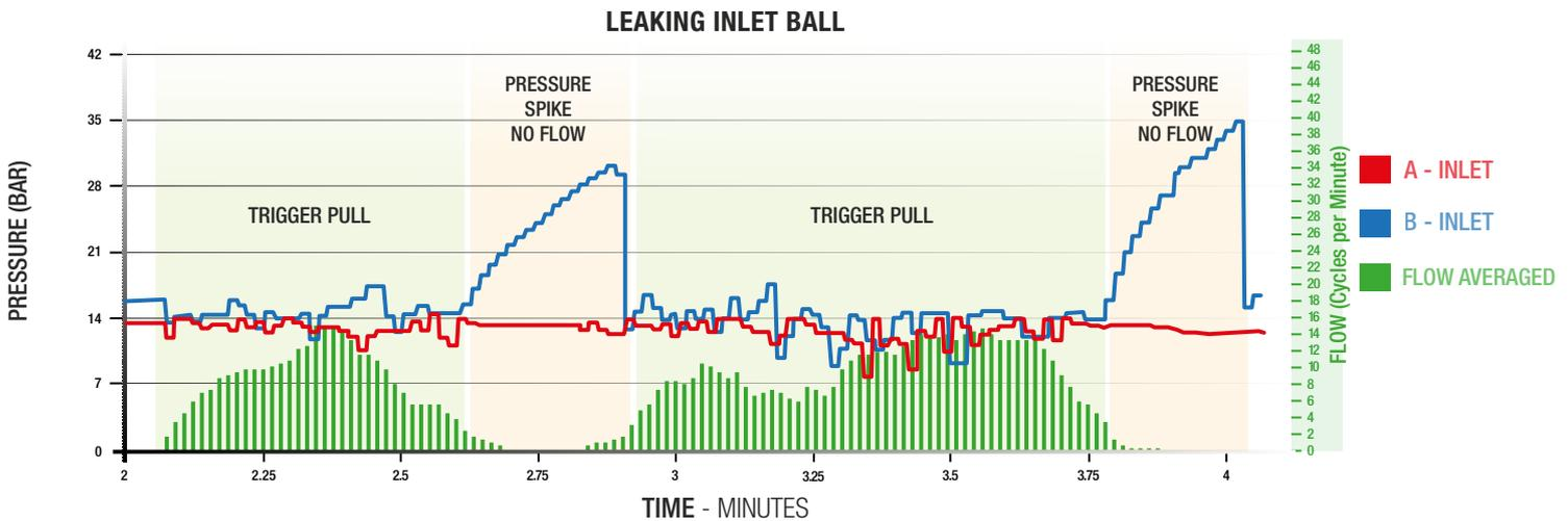
**Figure 8:** Graph shows pressure spikes on the B inlet during periods of no flow. The pressure spikes indicate an issue with the proportioner pump foot valve not resisting fluid pressure.
