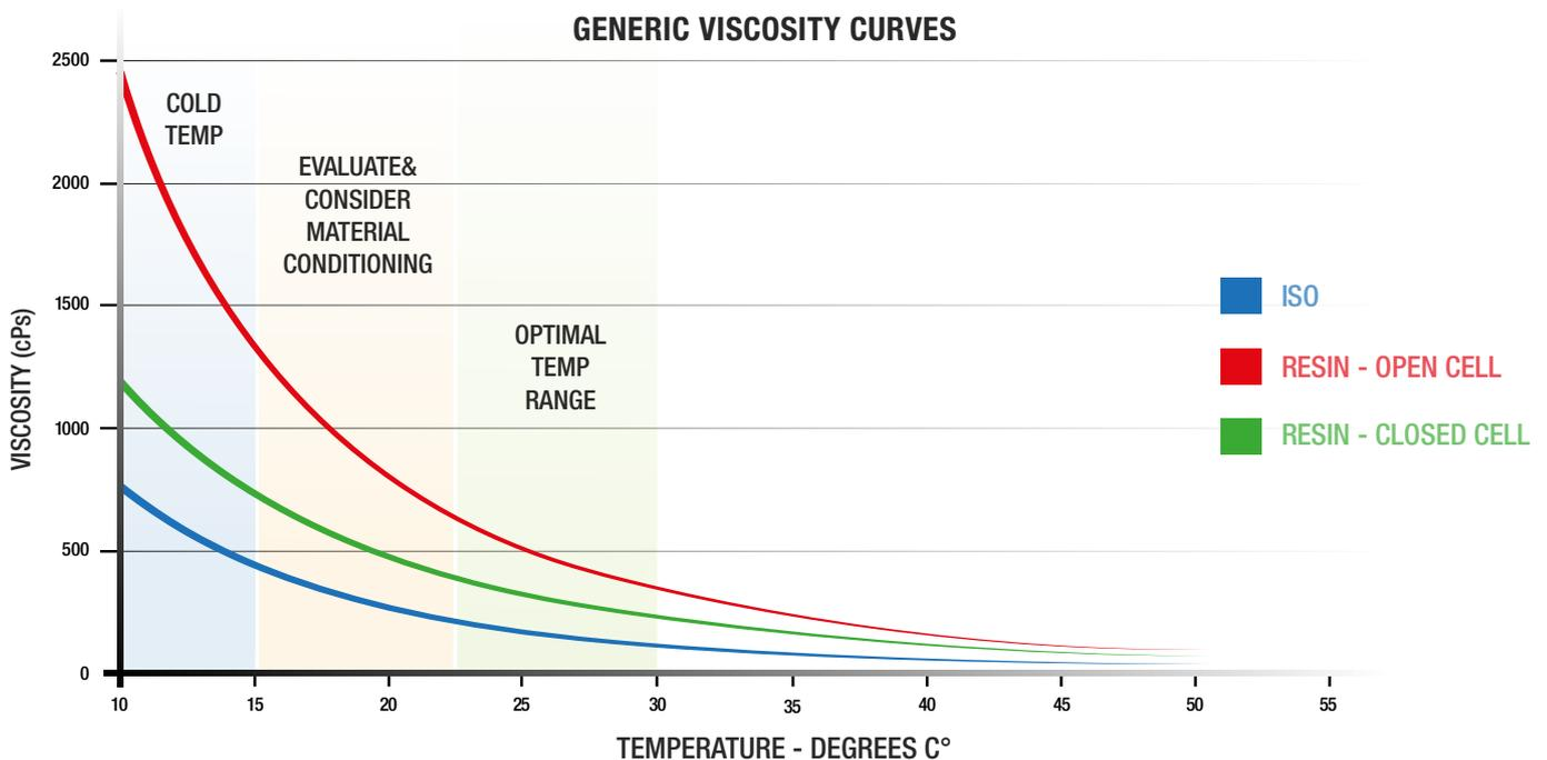
**Figure 7:** Graph shows how viscosities are affected by temperature. At temperatures less than room temperature the viscosities quickly increase which may cause feed pump issues. The graph is a generic representation for spray foam chemicals. Viscosities of actual materials used should be verified with the chemical manufacturer.
