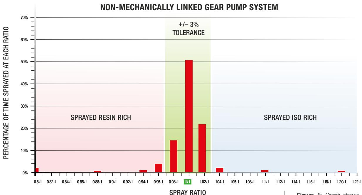
**Figure 4:** Graph shows actual spray data of a non-mechanically linked gear pump proportioner. The system dispenses outside of the 3% tolerance over 10% of the time. The ratios were calculated using a 1000 cc averaging window.
