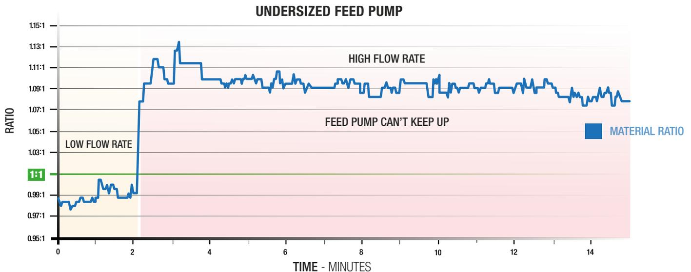
**Figure 6:** Graph shows that when spraying at a low flow rate the ratio is close to 1:1, but when spraying at a high flow rate the feed pump cannot keep up causing off-ratio spray between 1.07-1.11: 1
