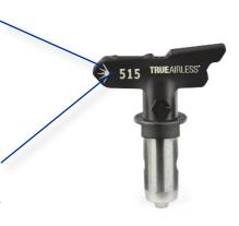
The orifice size defines the amount of paint that will flow through the tip. It is indicated by the last two digits: 15 in this case corresponds to a hole size of 0.015 of an inch or 0.38 mm. Your actual flow rate will depend on your spraying pressure and the paint you are using: high pressure - equals more flow; heavier paints equal less flow.
