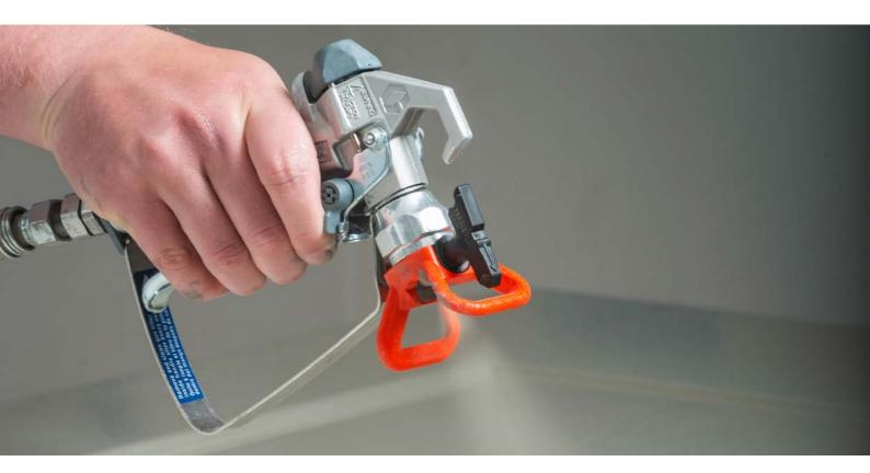
The spray tip tells the pump how hard it must work in order to maintain the required pressure. It ensures that the paint atomises under a certain fan width and flow rate — an effect similar to placing your thumb on the end of a garden hose.
