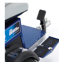
Dual Foot Pedal System (Patent 6,883,633)
