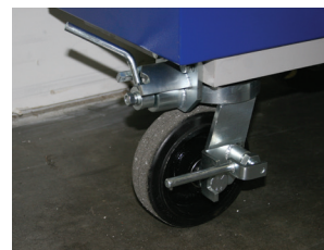
Rear Wheel System with release and brake.
