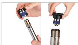
1) Insert pre-oiled packing cartridge assembly
