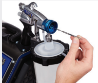
3) Pull needle out to release needle
