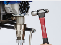
1) Loosen the clamping nut
