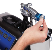
1) Remove front air cap and nozzle
