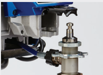
2) Open door and remove pump
