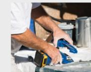
2) Remove the old pump from the sprayer
