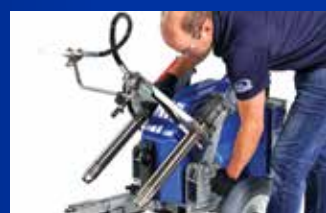
2) Tilt pump assembly back
