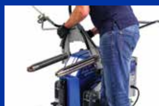
3) Remove ProConnect Pumping System
