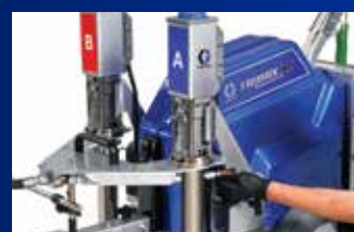
1) Remove retaining clamps and pressure transducer connections
