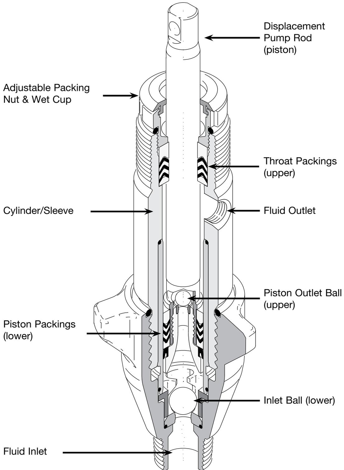
The general purpose of the packings is to create a seal and direct fluid flow. There are two sets of packings, **throat** and **piston**:
