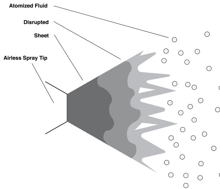
energy necessary to overcome the fluid's viscosity (resistance to flow) and surface tension (a force that bonds the surface of a liquid together) to form a fine spray.
