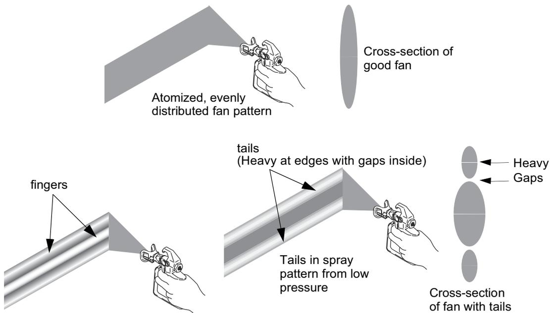
**Note:** If the maximum pressure of the sprayer is not enough to achieve a good spray pattern, a spray tip with a smaller orifice should be used. To test the quality of the spray pattern, test patterns should be sprayed on scraps of cardboard or other waste material.
