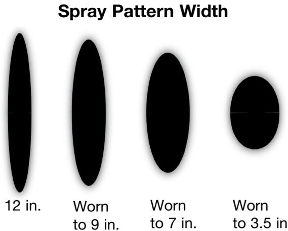
Example: When a tip that had a 12-inch fan pattern is reduced to a 9-inch fan when worn, it will output 40% more paint on 25% less area. Overlapping to achieve a consistent mil thickness becomes impossible. The chart above illustrates the effects of a worn tip on a spray pattern.
