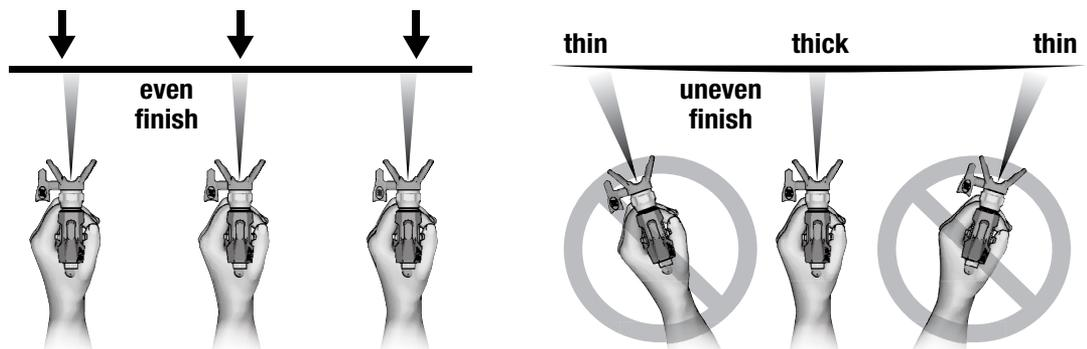
The spray gun should move across the surface with the wrist flexed to keep the gun pointed straight at the surface. “Fanning” the gun to direct the spray at an angle will cause an uneven finish.
