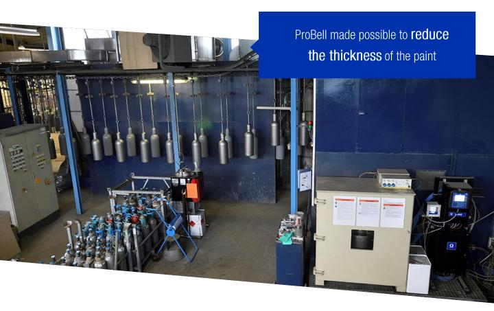
repeatable, uniform paint application on the rounded contours of the cylinders, thus achieving a uniform and correct coating thickness. This is vital. An overly thick coating could create problems during ultrasonic testing of the cylinders.
