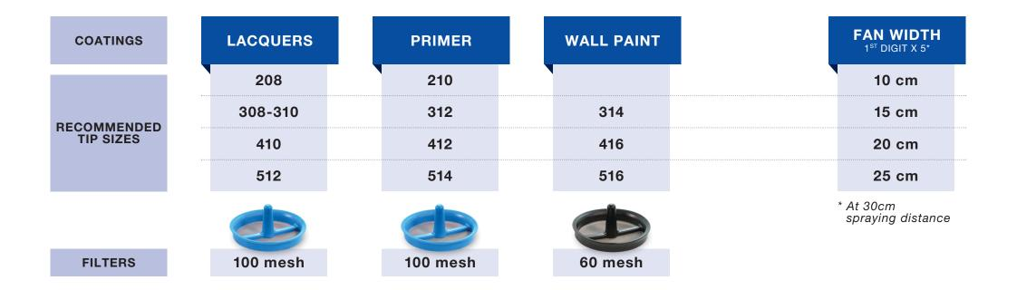
For proper sprayer operation use only FFLP tips, the same tip family delivered with the Ultra<sup>®</sup> QuickShot<sup>™</sup>.
