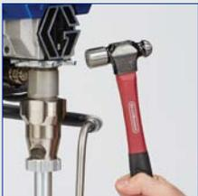
Loosen the clamping nut
