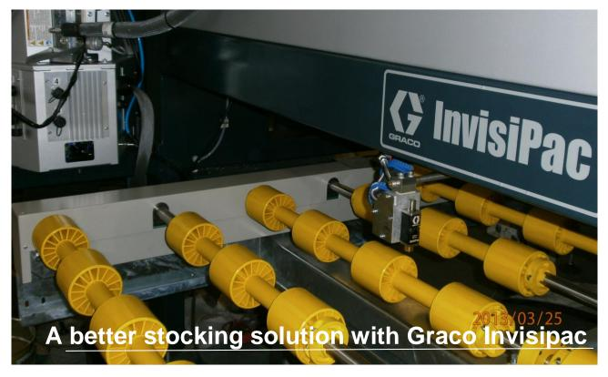
The company Grupo Palazon y Mira, in Alicante, Spain, produce and stock marble slabs. To avoid a vacuum effect when stocking the slabs one against another, they were introducing a piece of paper between the slabs. They needed a new and easier solution to stock their marble slabs, one which would keep air circulating between the slabs to avoid the vacuum effect, reducing manual work and damage to the marble.
