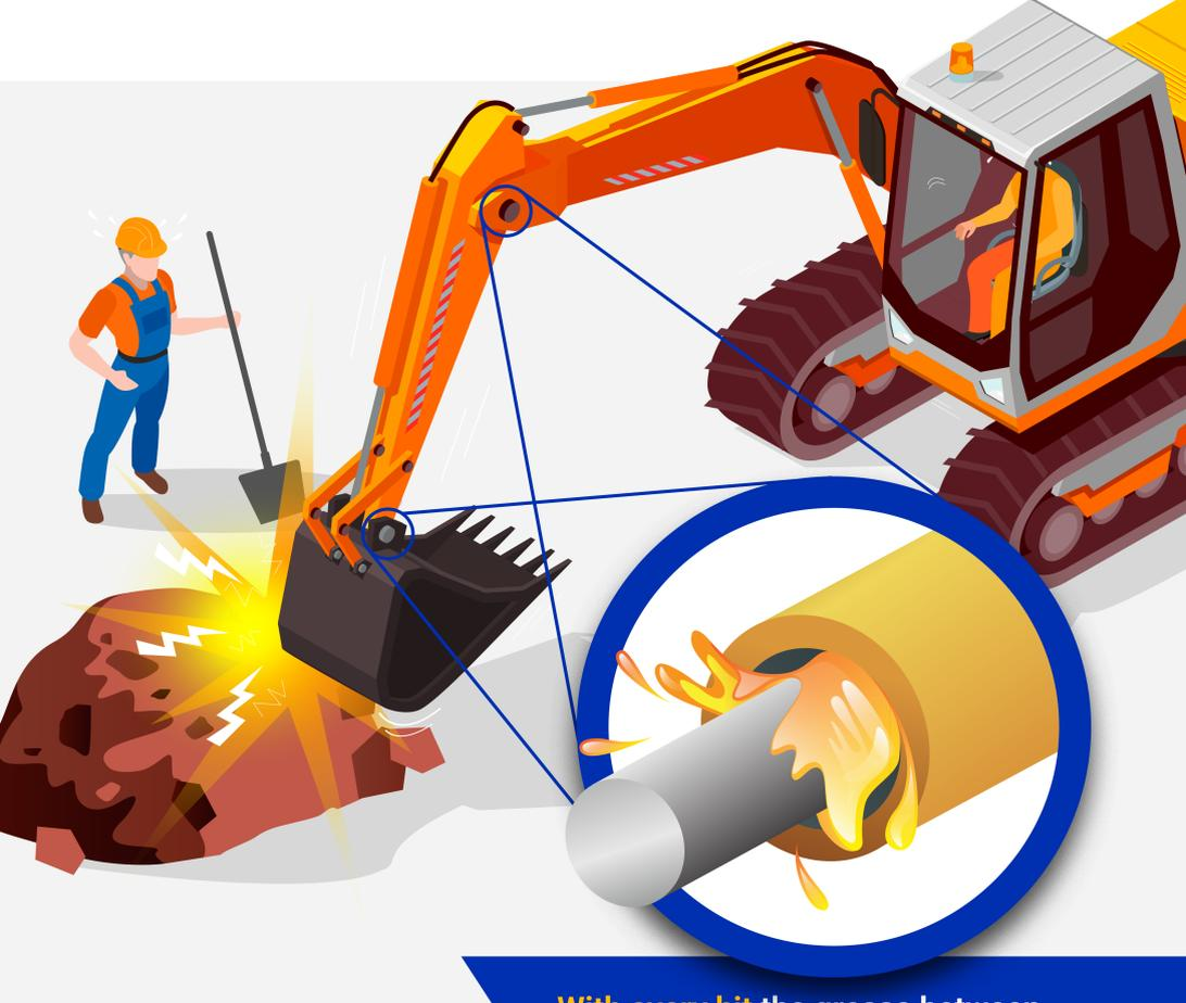
With every hit the grease between the pin and bushing is squeezed out, creating **metal-to-metal contact**
