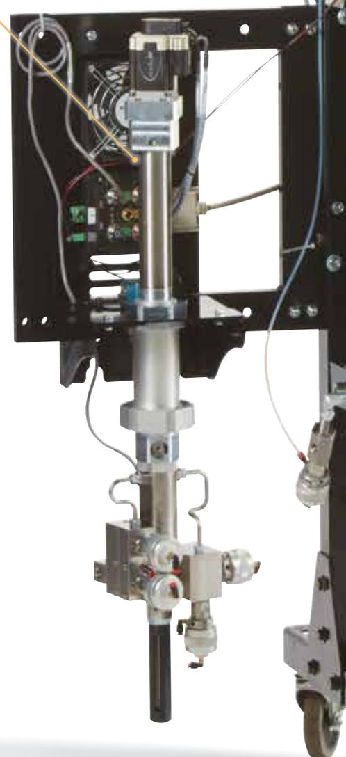
“*The ProMix PD2K is easy to set up and maintain. It handles various inbound pressures and viscosities without touchy fine-tuning, and pumps can be rebuilt in less than 20 minutes.*”
