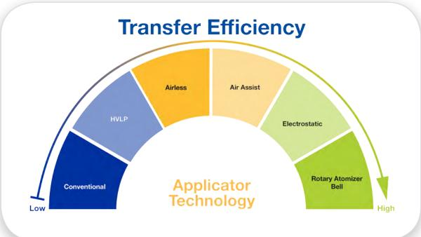
Transfer efficiency is the amount of paint solids deposited on a part divided by the total paint sprayed. Look for the colored boxes next to each gun type to see how our guns stack up.
