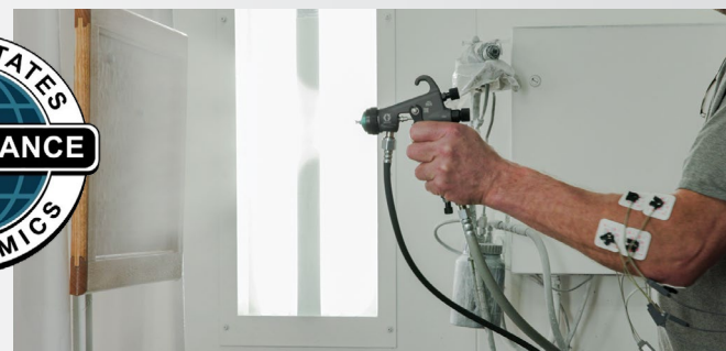
Testing shown involved spraying water during muscle effort monitoring by United States Ergonomics.
