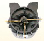
Load Minimizing Drive Each G3 piston pump element is offset from the main motor shaft resulting in less stress on the motor and internal components.
