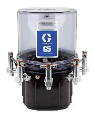
Offered either as a standalone pump or within an enclosure, the Graco G5 can be customized to meet your application standards. Enclosures are available in two sizes — the larger can house an optional auto-fill shutoff (AFSO) and pressure relief valves (PRV) whereas the smaller enclosure can house just PRVs with the pump.
