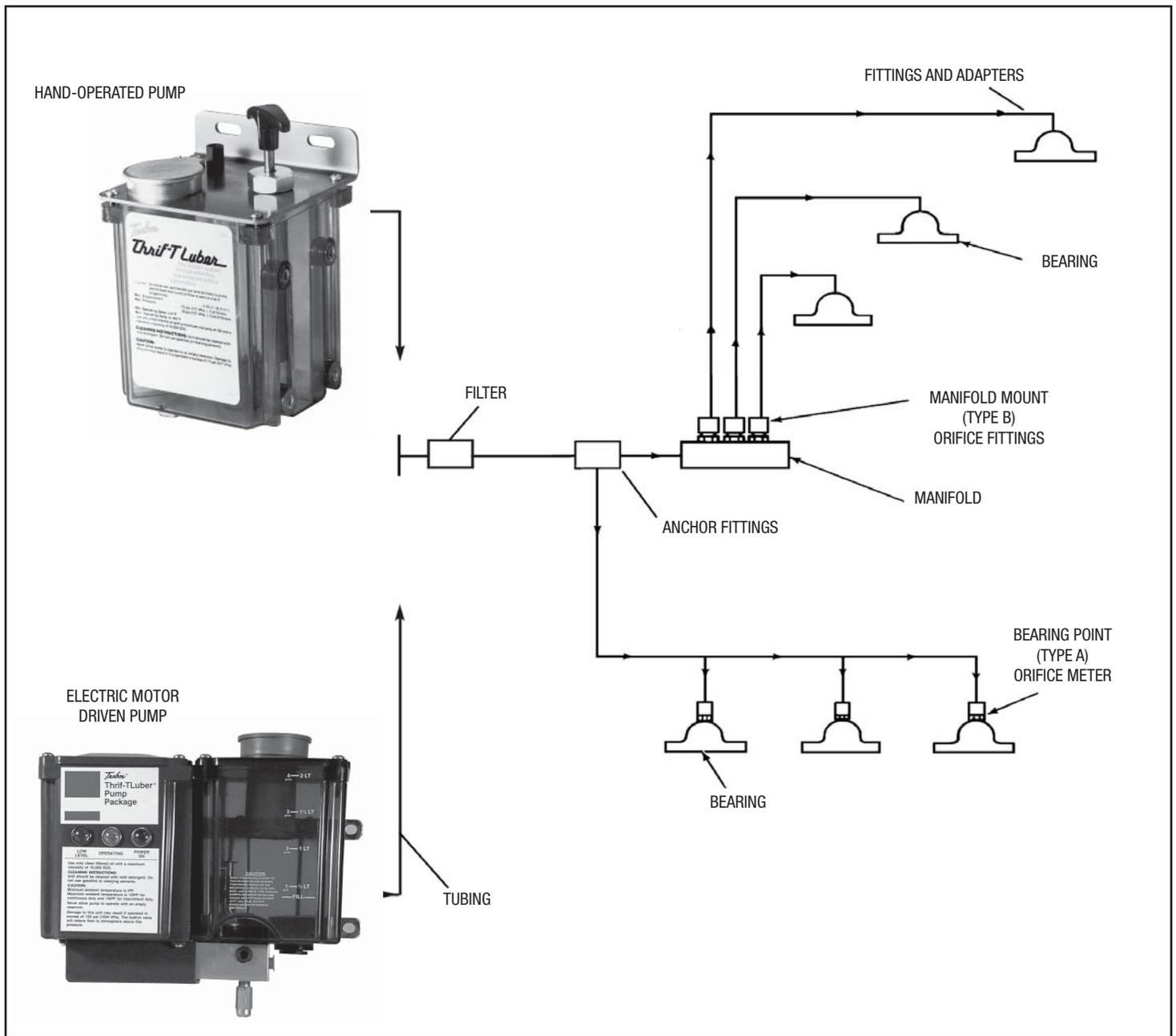
Figure 1: Thrif-T Luber System Diagram
