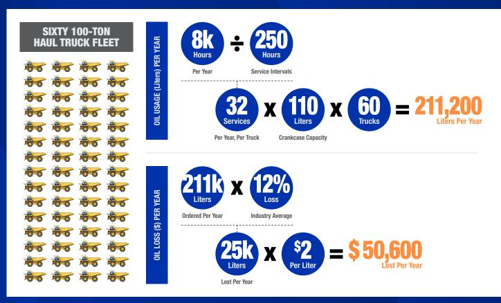
While already a substantial expense just quoting for the haul truck fleet, we can logically extrapolate using these numbers to see the magnitude of oil expense across a mining site's heavy equipment. The loss of oil, which amounts to 12% of the initial purchase volume, amounts to a tremendous waste of capital that can be reinvested into the business.
